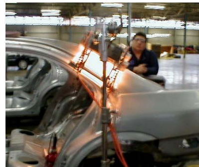
Figure 2: Infrared Line Heater installed at Ford Motor Company for epoxy curing
