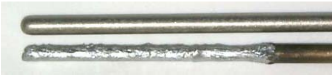
Figure 2A. Thermocouple sheaths after being exposed to molten aluminum; Lower probe is uncoated after 91 cycles.
