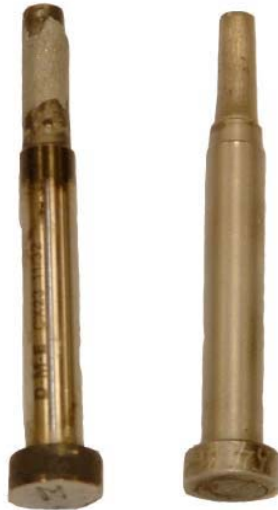
Figure 1. Untreated and treated H-13 steel die pins after 3,500 and 200,000 shots of aluminum respectively
