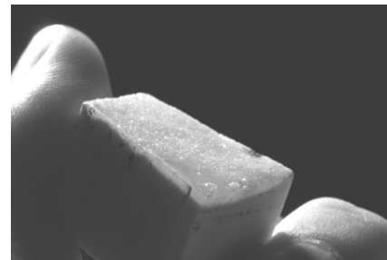
Photo of nozzle surface melted using ORNL high-intensity IR lamp
