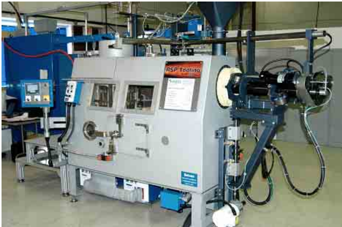
Figure 4.1 The beta RSP Tooling machine constructed by Belcan Corporation for RSP Tooling, LLC
