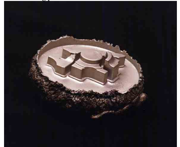
Figure 1.1 A close look at the GMTI Die from the RSP Tooling process
