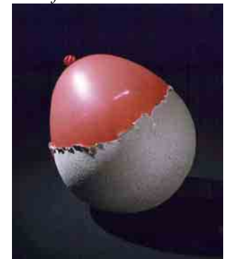
Figure 1.2 This party balloon covered with tin alloy demonstrates the abilities of rapid solidification
