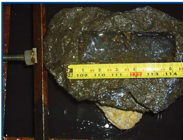
Sample after the run, showing the kerf cut by the jet
