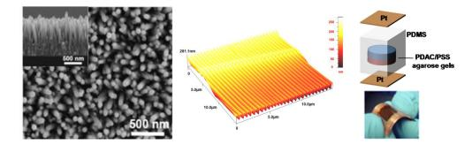
Left: Scanning electron micrograph (SEM) of zinc oxide (ZnO) nanorod growth by a combination of hydrothermal and atomic layer deposition techniques (cross-section SEM inset). Center: Atomic force micrograph of a buckled nanostructured substrate with an indium tin oxide (ITO) coating for use in an organic solar cell device. Right: Prototype of a new flexible gel-based photovoltaic device.
