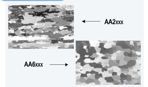
**M**icrographs showing the microstructure evolution after hot rolling and annealing of alloys AA2xxx (AI-Cu-Si-Mn) and AA6xxx (AI-Si-Mg).
