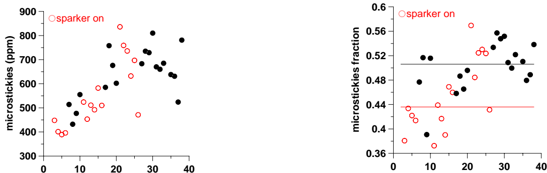
Figure 3: Effect of sparking on cleaner efficiency. Microstickies are shown on the left panel. The microstickies fraction is displayed on the right.
