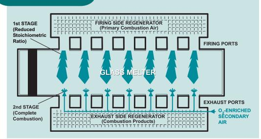
$\mathbf{O}$ xygen-enriched air staging uses a two-stage process to reduce NO<sub>x</sub> formation.
