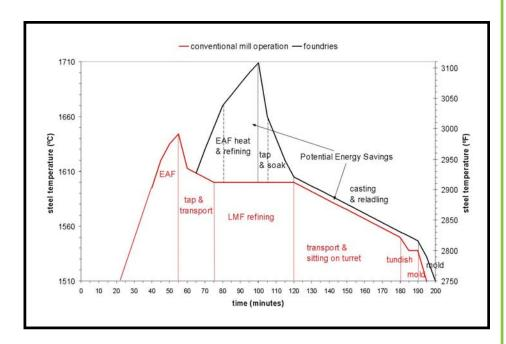
The temperature-time history of a heat of steel in a foundry and a mini-mill. The area under the curve conceptually illustrates the energy usage. Best practices in the foundry should eventually approach the mini-mill.
