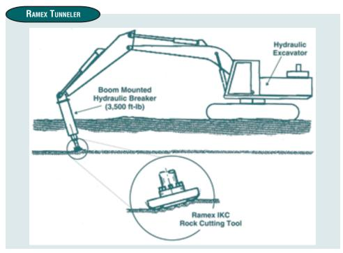
Foundation and/or trenching excavation system used to field test the Ramex IKC rock cutting tool.
