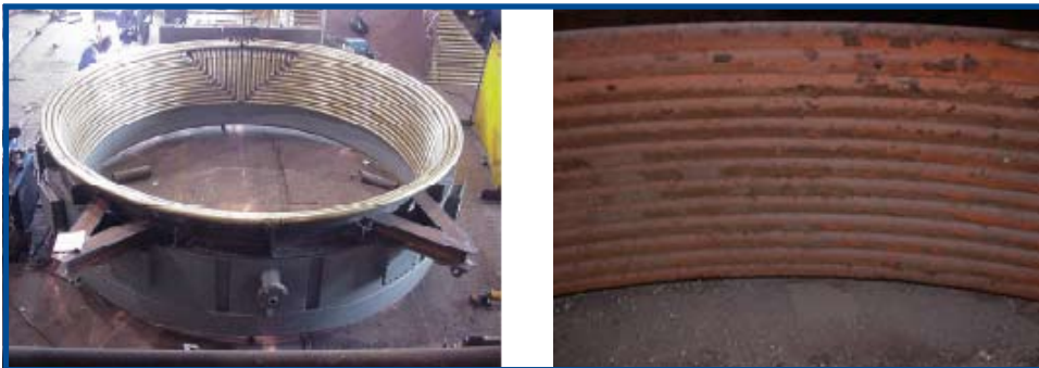
Photos of aluminum bronze skirt prior to installation (left) and after 4,563 heats (right). As of June 2007, the skirt has processed about 6,000 heats without requiring process-related maintenance, compared with traditional skirts that typically require some maintenance after only 80 heats.
