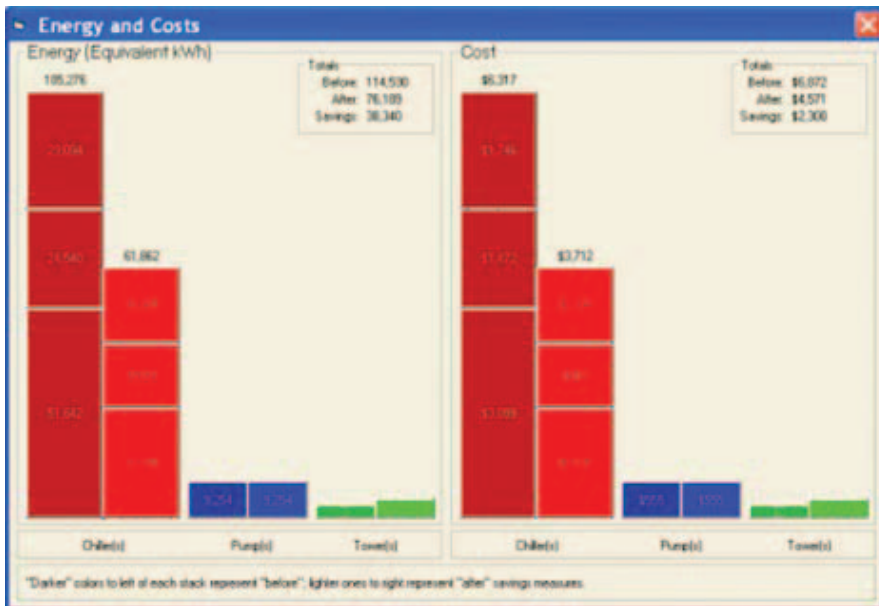
Figure 2: A sample "before and after" graph of a chilled water system's energy consumption and costs. (Note: In this example, the effects of decreasing condenser water temperature are being analyzed).
