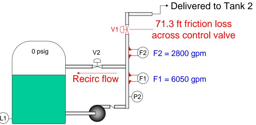
Required flow rate: 2800 gpm sent to Tank 2
