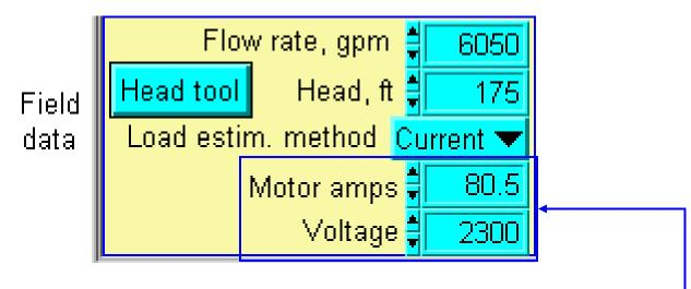
Either motor current or power can be used to estimate the motor shaft load
