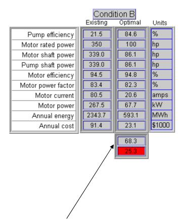
Optimal equipment sized to meet the <u>required</u> conditions could save over \$68,000/year.
