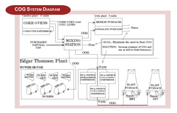
and reheat demand vary significantly over time. In most plants, during periods of low electric, steam, and reheat demand, some COG has to be flared because there is no use for it. Recognizing the flared COG as a valuable source of energy and cost savings, USS developed a project to utilize it.
