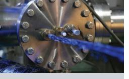
Dow is working with DOE's Oak Ridge National Laboratory to produce highstrength carbon fiber using polyolefin, a low-cost plastic.
