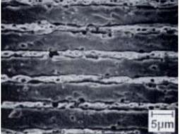
Fabrication: Tape cast layers w/ screen printed electrodes
