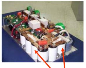
Electrolytic capacitors cannot meet the 110°C requirement for DC Bus Capacitors for 2004 Electric Hybrid Vehicles:
