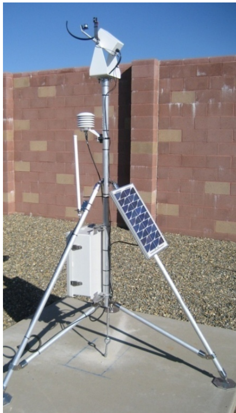
Figure 9. Solar monitor / meteorological station
