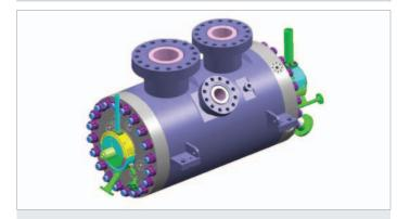
This project's team will build a prototype of the largest and highest-temperature s-CO<sub>2</sub> closed Brayton power cycle turbine ever constructed. The use of carbon dioxide instead of steam allows higher power-cycle efficiency and more compact cycle components. *Illustration from Dresser-Rand*
