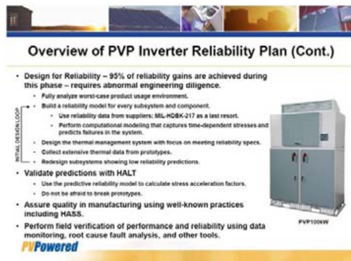
Figure 8: Features of PVP Inverter Reliability Plan
