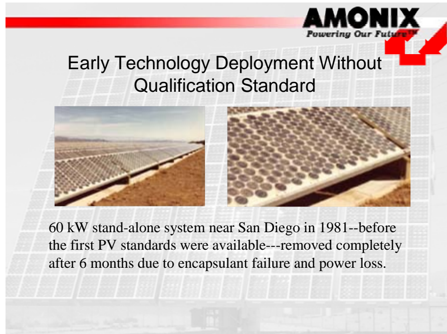
Figure 11: Early CPV Example Without Qualification Standard
