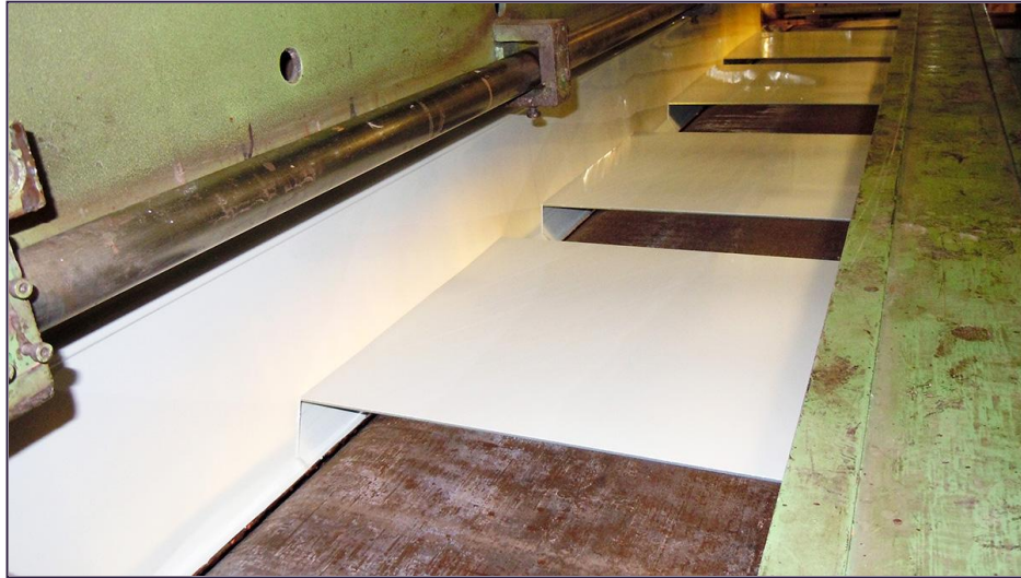
17.5 inch x 72 inch full-size mirrors passing through curtain coater
