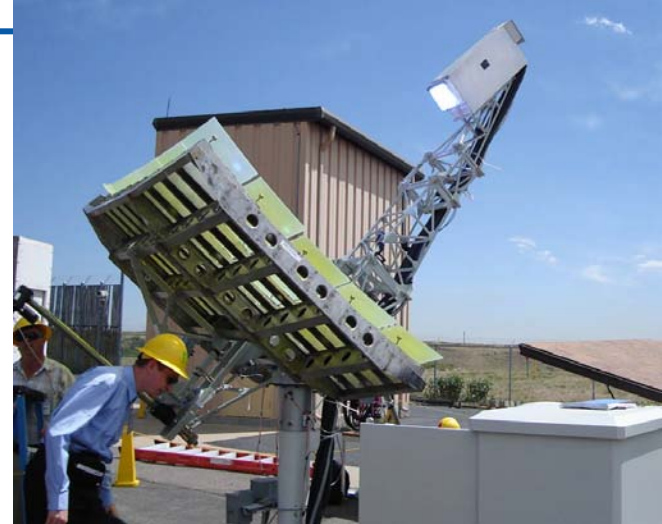
New UV dish includes environmental chamber; same 100X < 500 nm, but 4x size
