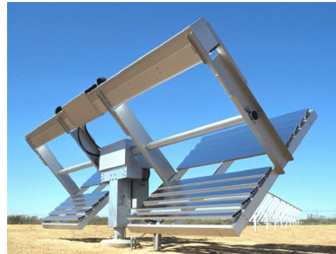
EMMAQUA: Phoenix, AZ X7 to 8 cooled—near ambient sprayed w/ DI H 2 O 8 min /nat. sun hr
