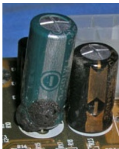
Figure 11: Example of a failed electrolytic
