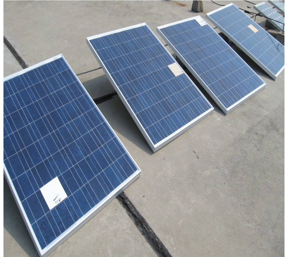
Long term hot spots testing on roof
