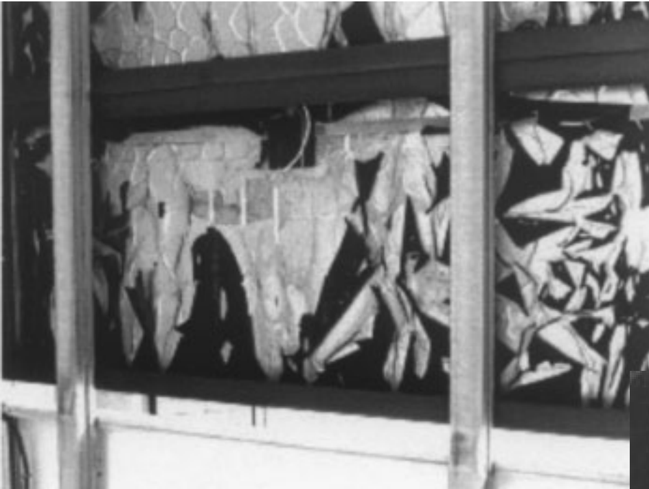
Backsheet crumbling (Italy; 22 years)
