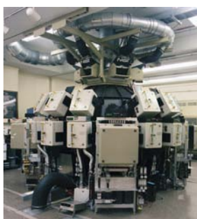
NIST-Patented 2-meter SPHERE (Simulated Photodegradation via High Energy Radiant Exposure) • Chin et al, Review of Scientific Instruments (2004), 75, 4951; Martin and Chin, U.S. Patent 6626053
