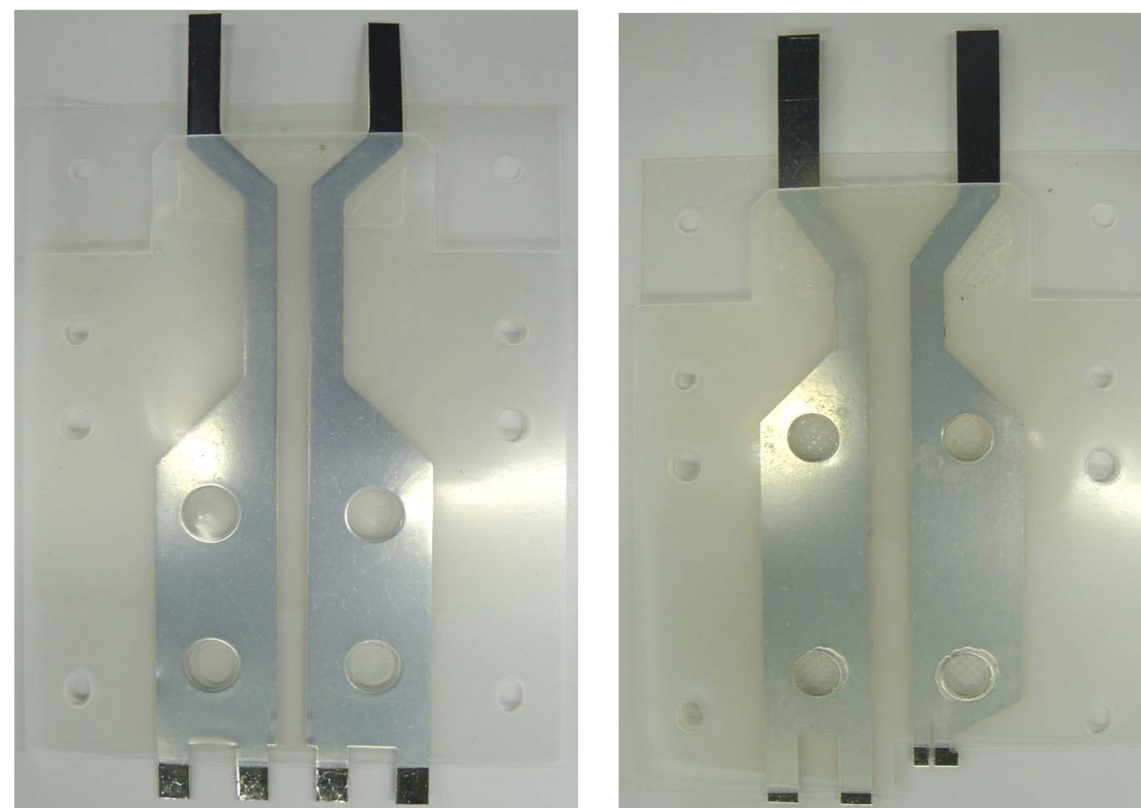
Figure 2. Two versions of Transform Solar's solder tail subassembly. Each of the individual module designs at Transform Solar have a unique tail configuration to accommodate the certification requirements
