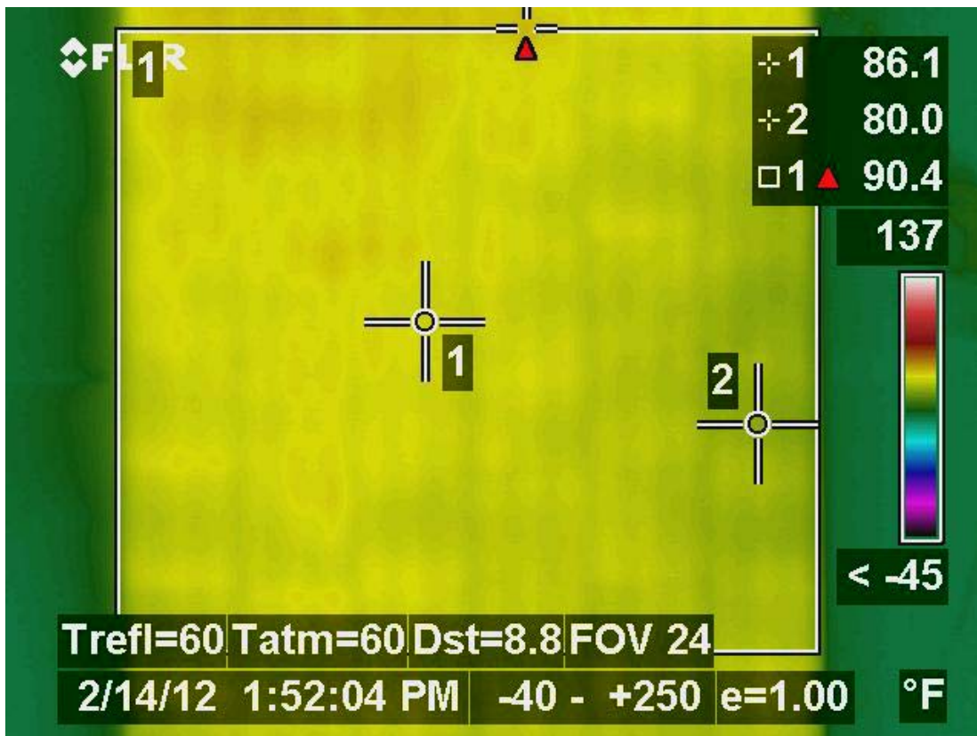
Figure 8. IR Image of 235 Watt Solar Module
