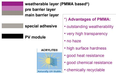
Perfect Transparency of PMMA for Solar Cells
