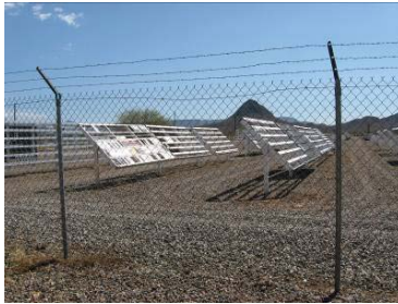
Static Racks (5° or latitude w/ backing)
