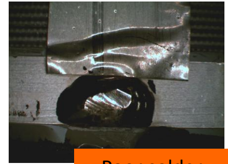
Poor solder joint wetting
