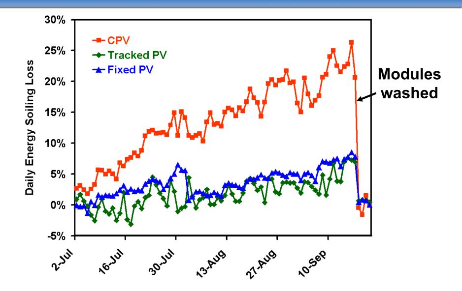
Dirt accumulation may be easily removed by small (0.8 mm) rain events
