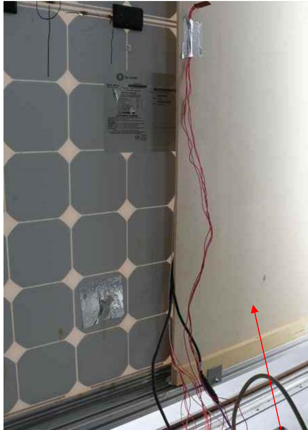
Back of module ( Sample B ) completely enclosed before start of test
