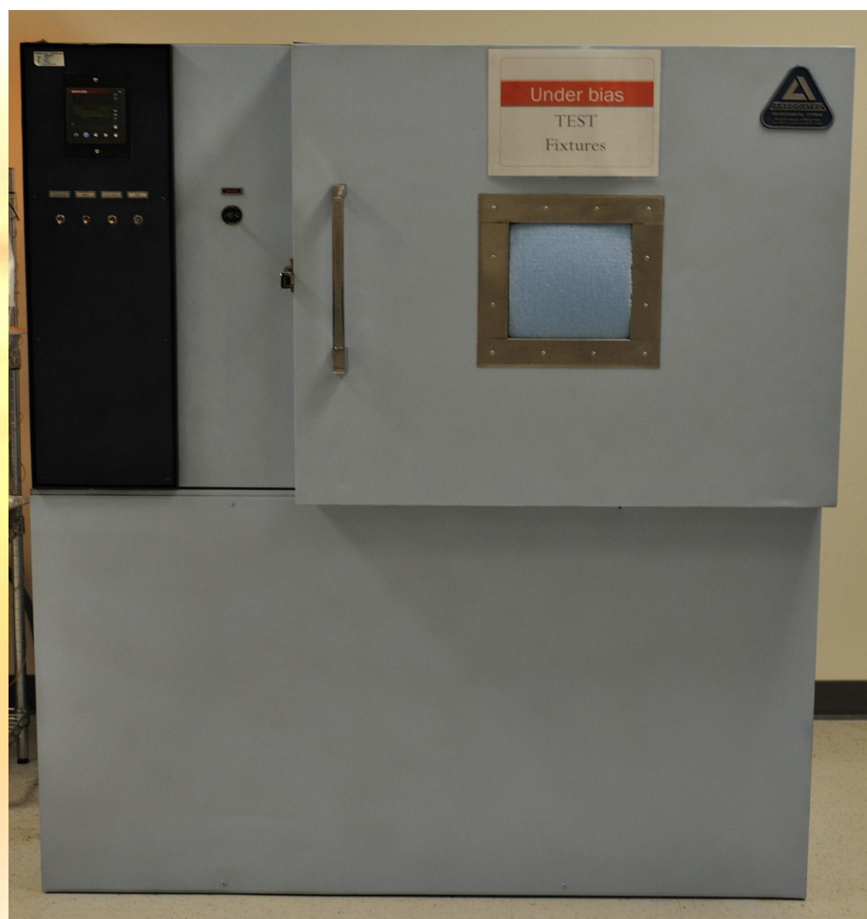
N.I.S.T. Cycling Chamber -40°C to 110°C
