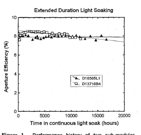
Figure 1. Performance history of two sub-modules fabricated using different recipes. The need for long term testing is apparent.
