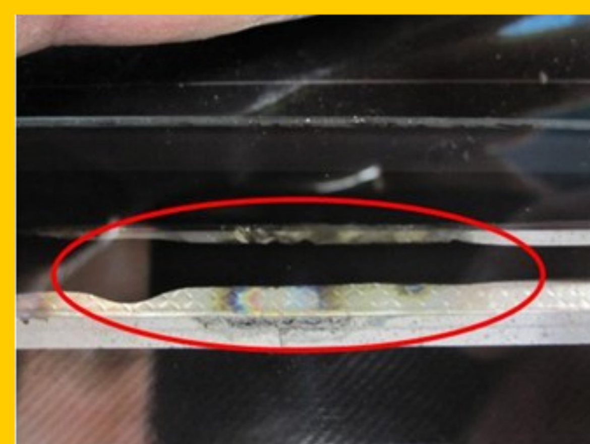
Buss tape failure as seen from the backside of the module
