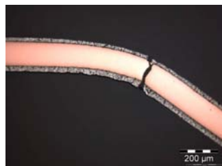
Fig. 1: broken copper ribbon [1]
