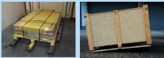
Figure 1 & 2: A complete shipping unit exposed to transport-like vibrations and handling induced shocks (rotational flat drop test)
