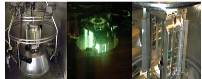
Customized testing instrument using an Atlas xenon Weather-Ometer for high-flux stress test of encapsulants for medium-concentration concentrating photovoltaic (CPV) system at National Renewable Energy Laboratory (NREL)
