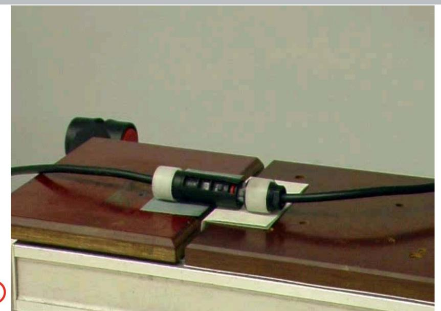
Strain from cable, birds and ice weight compounded by sway and leverage of the cable strain relief gland.
