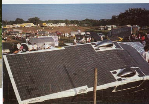
Crowder's "Star II" is tilted toward the sun to help recharge its batteries on the morning of the second day in Floral City, Florida.
