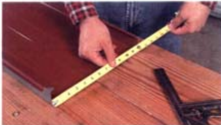
This panel is only 12 inches wide – obviously not an acceptable profile.
