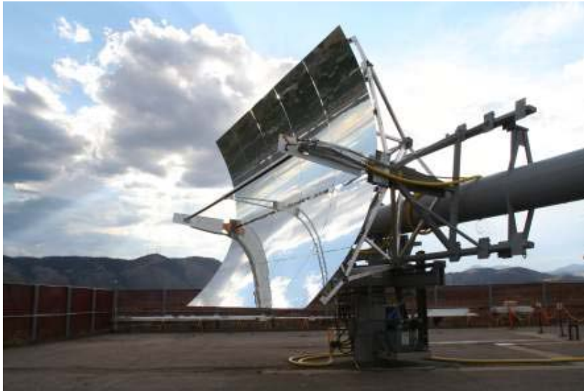
Optical efficiency testing on 2-axis tracker
