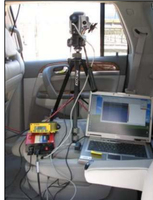
Camera and GPS for exact positioning
