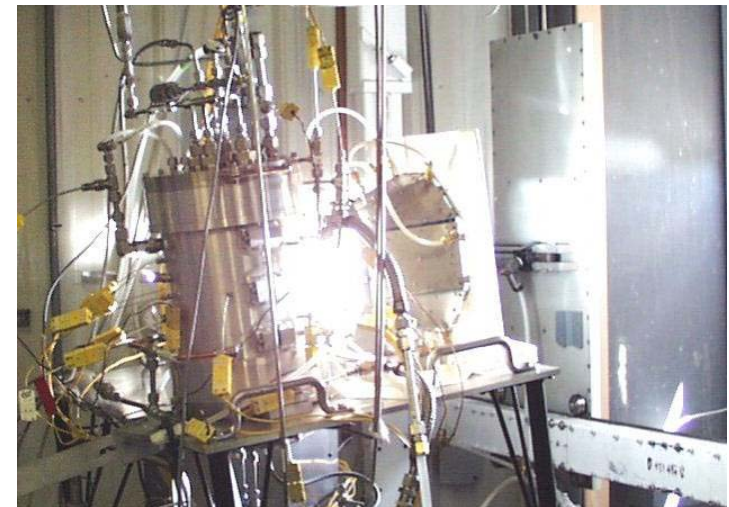
Applications include high-temperature thermochemical reactions and small Stirling engine and CPV performance testing
