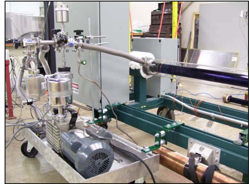
Comparison of UVAC3 and UVAC2 Heat Loss NREL Thermal Test Bed - March and October 2007 Information regarding testing available at: http://www.nrel.gov/csp/troughnet/testing_standards_reports.html#receivers
