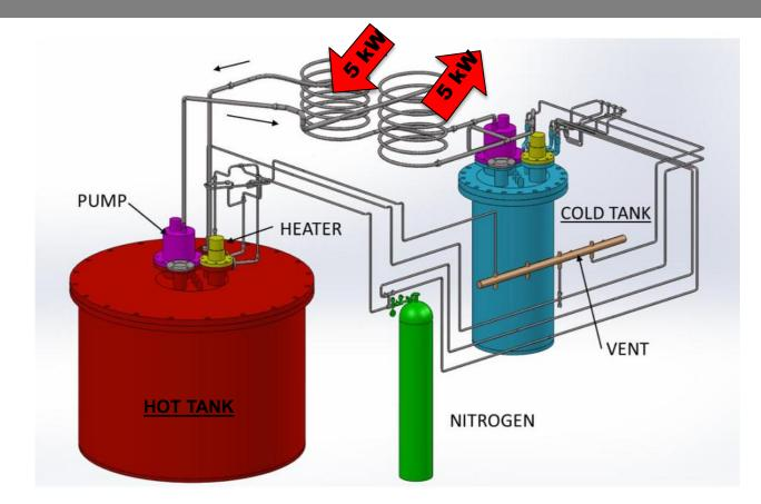
• Pilot scale thermal storage system (30 kWh, 400 kg glass)
