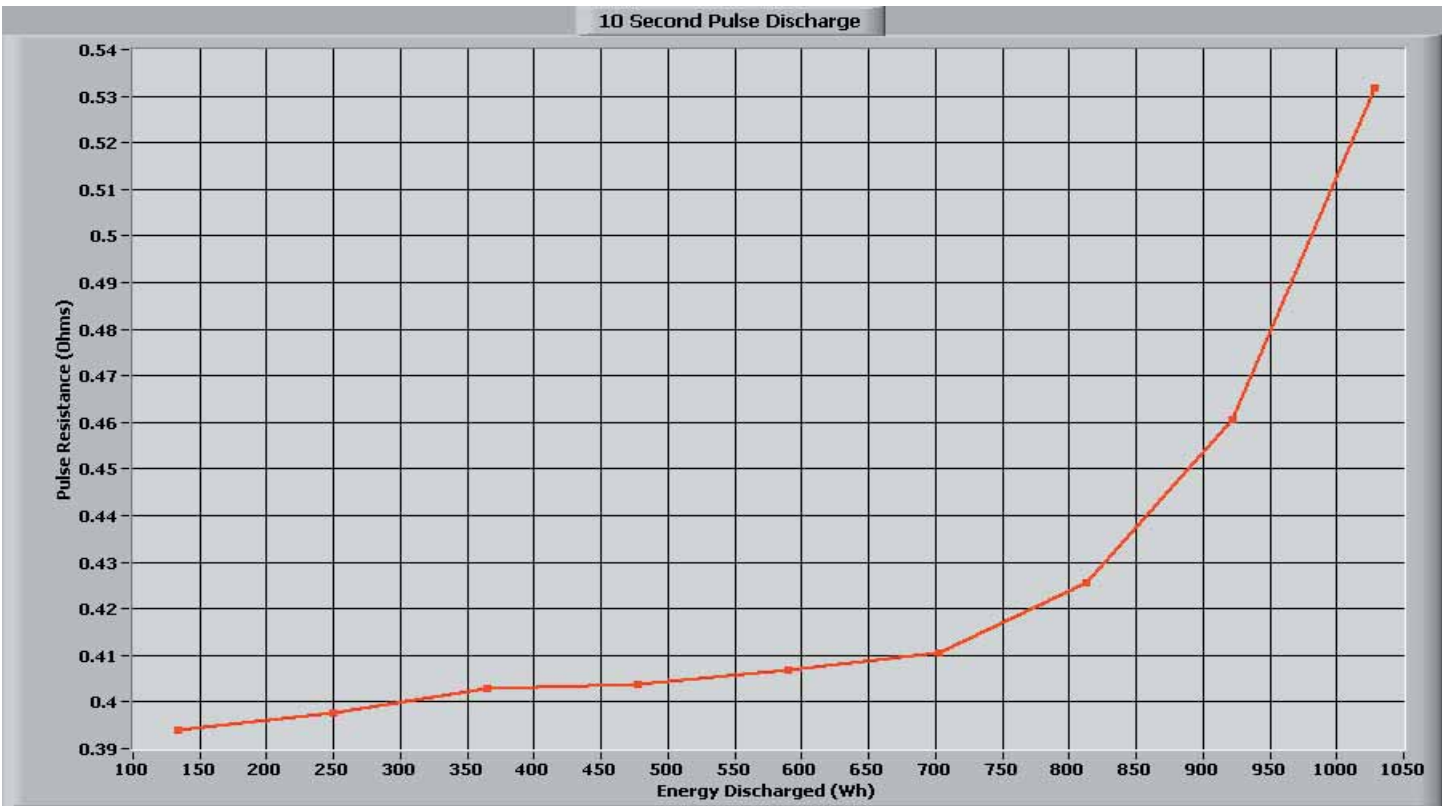
Figure 4 Discharge Pulse Resistance vs. Energy Discharged
