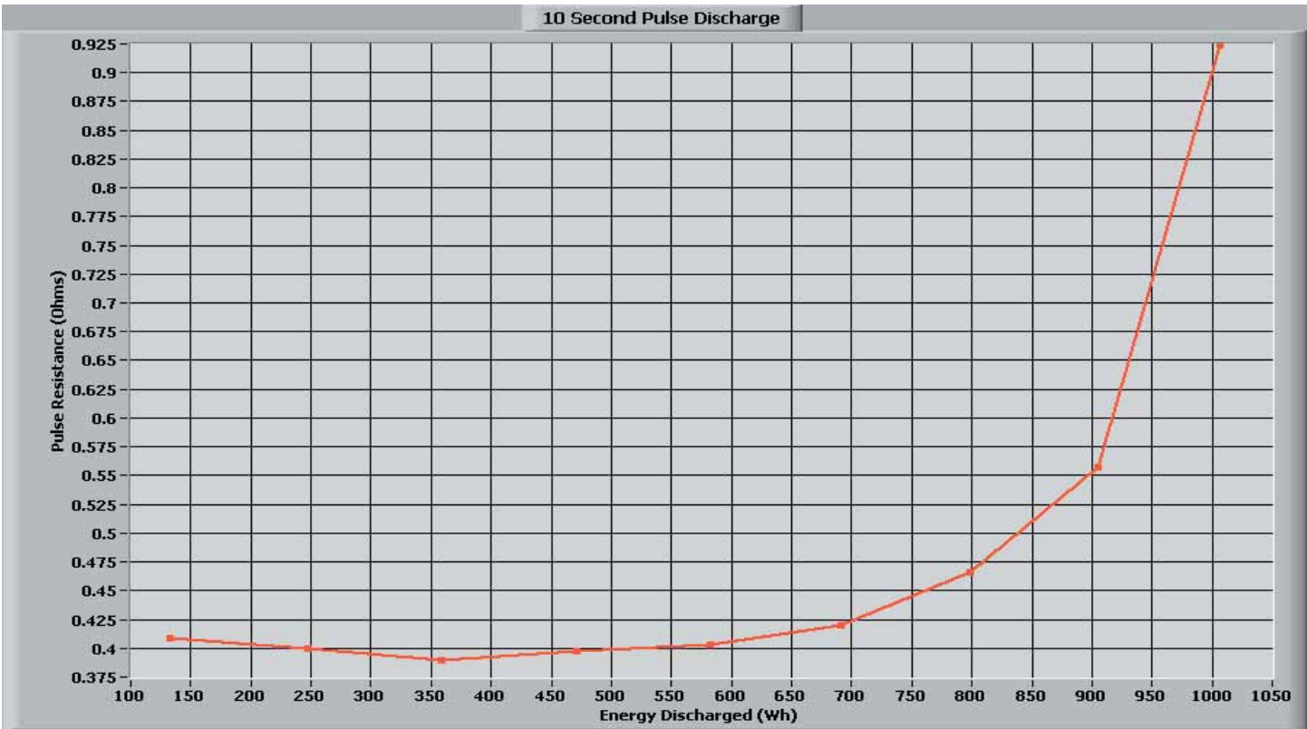
Figure 4 Discharge Pulse Resistance vs. Energy Discharged
