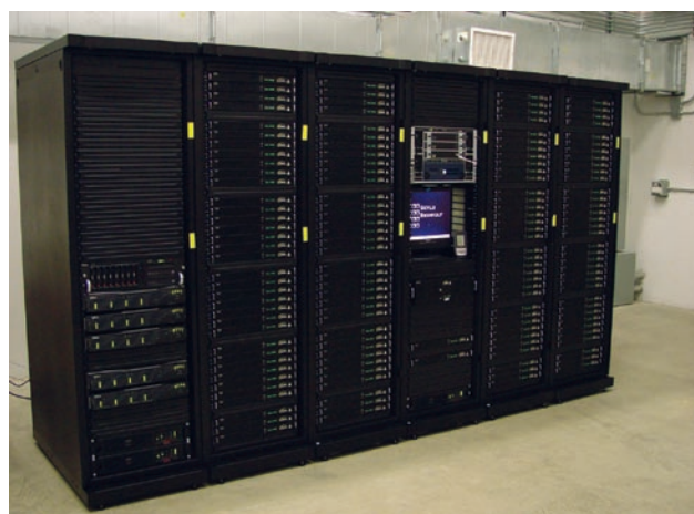
FIGURE 3. Baseline cluster configuration housed at Sandia National Laboratories (284 AMD Opteron™, Model 246, 2.0 GHz) processors with InfiniBand interconnect and 20 terabytes of RAID 5 disk storage.
