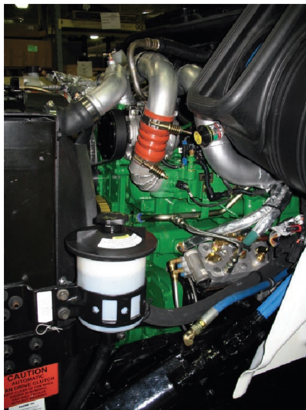
FIGURE 6. View of Truck Showing Deere 9L Engine in 8600 International Truck
