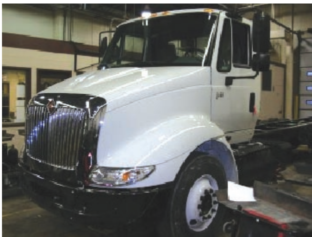
FIGURE 7. Truck Running on NREL Chassis Dyno
