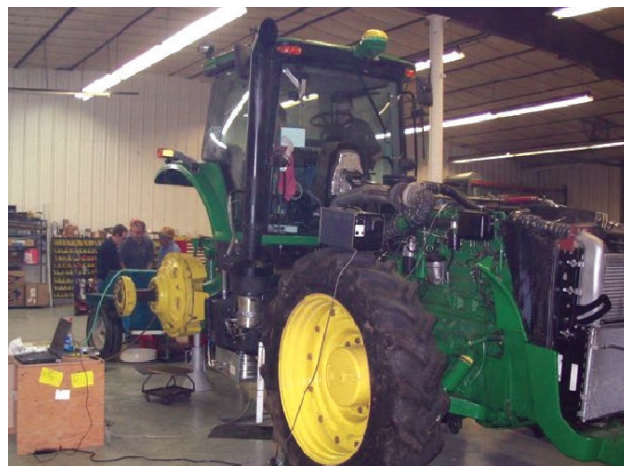
FIGURE 5. Turbo Compounded 8530 Tractor on Dyno
