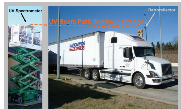
FIGURE 1. Picture of the UV remote sensing technique being deployed during a field campaign at the I-40/75 weigh station.
